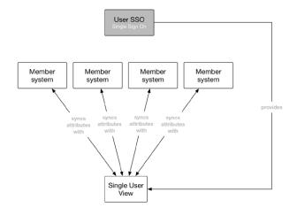
The diagram above describes how the Single User View is provided by the directory service provided by the SSO product and how it interacts with the various member systems it is connected to, detailing two way attribute synchronising
